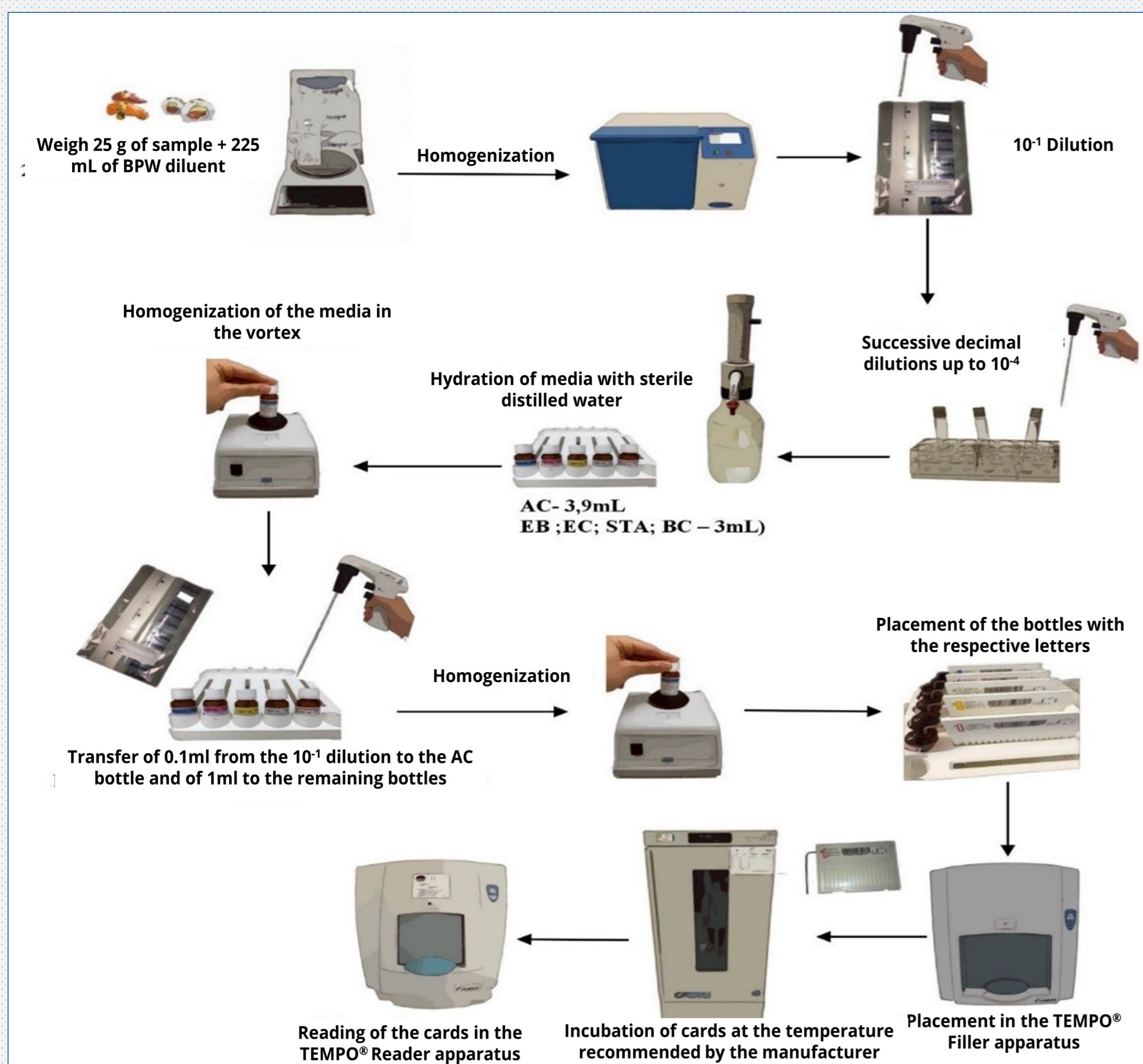
Fig. 1. Schematic illustration of the procedure for searching for AC, EB, EC, STA and BC using the automated method (From Alegria et al , 2020).
